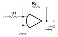
Gain = feedback resistor  $\div$  input resistor or Gain = 470  $\div$  10 or 47
