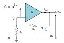
The gain of an operational amplifier is controlled by feedback resistor that can very accurately control the gain of the amplifier in a circuit. In the circuit shown below the gain is determined by the ratio of the input resistor and the feedback resistor.
