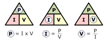
The power law describes the relationship between Voltage in Volts, Current in Amperes and Power in watts in a circuit. The triangles shown above allow you to easily determine the unknown when the other two quantities are known,
