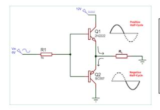
This is a class B push pull amplifier output stage. Each transistor only conducts on one half of the cycle, but they are summed to produce a full cycle. The advantage over a class A amplifier is that there is little or no current flowing when there is no input signal. There will be some loss of signal at the crossover point which will show up as distortion.
