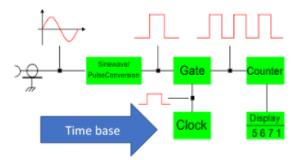
The gate open time is determined by the time base, which determines the time over which the incoming signal is counted.
