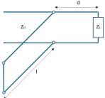
Stub matches are widely used to match any complex load to a transmission line. They consist of shorted or opened segments of the line, connected in parallel to a line at appropriate distances from the load. The single stub match is a widely used matching circuit.
